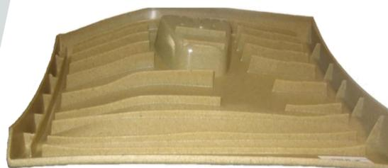
Figure 12: In combination with CADMOULD Fiber, CADMOULD Warp also takes fiber orientation into account. The accuracy of warpage results is shown here for the example of a glove compartment (top half), for a natural fiber reinforced material. Combining Warp with VARIMOS brings the additional benefit of being able to optimize warpage with automated methods.
