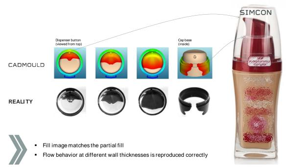
Figure 7: CADMOULD was used to simulate this cosmetics bottle spraying nozzle, for L'Oréal Paris. The challenge with this kind of part is that there is a variety of wall thicknesses. There is a very thin connection between the base of the cap, and the cap itself, and there are thicker parts before and after. The results show: filling behavior matched the partial fill perfectly.
