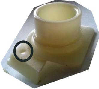
Measured sink mark depth: **0,25 mm**
