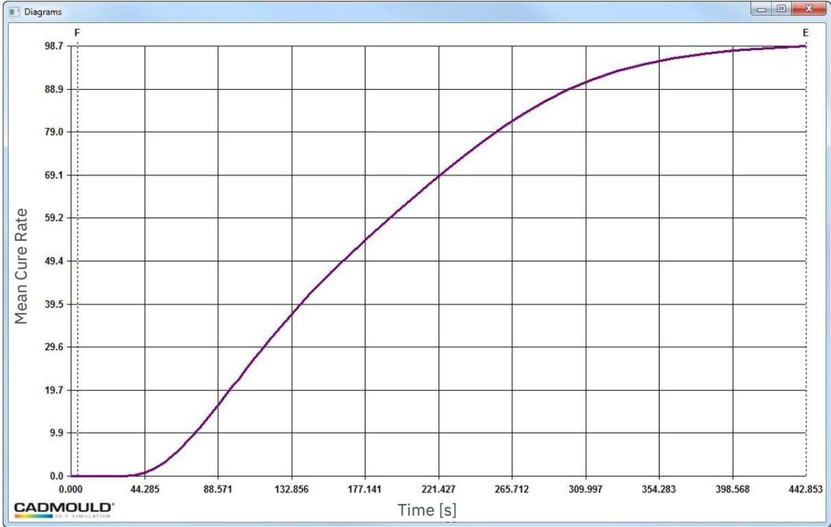
Figure 25: CADMOULD Rubber, displaying the evolution of the mean cure rate across time
