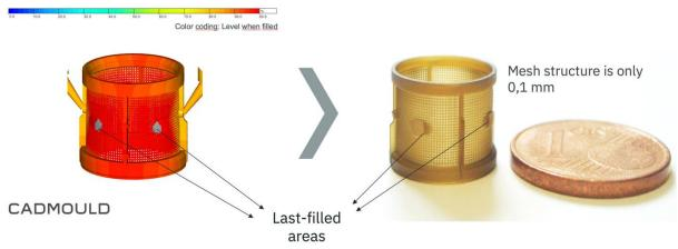
Figure 6: CADMOULD Fill was used to simulate filling of this filter, used in an ABS brake system for a car. CAD-MOULD was used to find the right places to put venting zones, in order to avoid filling issues in the filter mesh. The simulation proved extremely accurate, even for this extremely thin / fine part. The elements of the filter mesh have a diameter of 0,1 mm and less.
