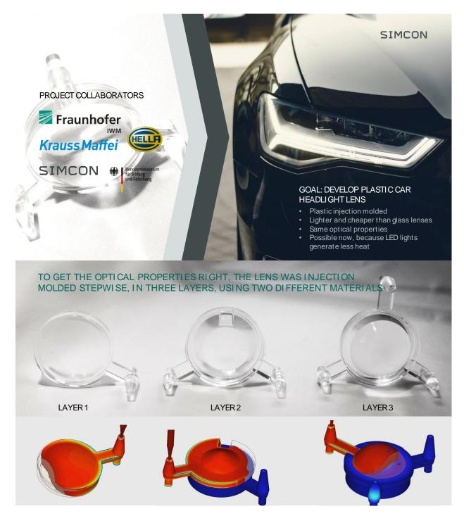
Figure 17: CADMOULD was used to simulate the filling of this complex, thick-walled, multi-layered, multi-material car headlight lens. This project was undertaken with our partners at Fraunhofer, Hella and KrausMaffei. For optical parts, precision is crucial. The 3K filling of both macro structures and Fresnel-type microstructures was simulated accurately.
