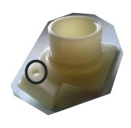
Simulated sink mark depth: 0,23 mm
