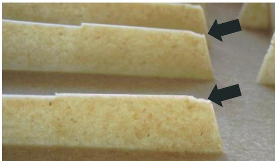
Figure 10: Accurate simulation of filling behavior for a fiber-reinforced material helps identify filling issues
